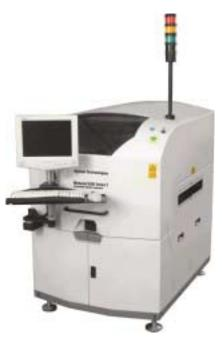
Flexible AOI detects and prevents defects at multiple stages of your production line.
