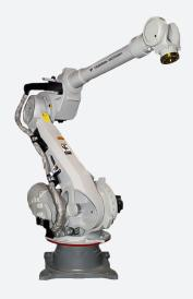
Developed for material and part handling, the Motoman MH165 robot does just that. A vertical reach of 3,372 mm and a horizontal reach of 2,651 mm give this MH165 DX100 industrial robot a large work envelope perfect for transferring parts. End of arm tooling can be stored behind the robot because of its large work envelope. Combine that with a payload capacity of 165 kg, the Motoman MH165 DX100 robot can be used in a variety of heavy industrial settings.
