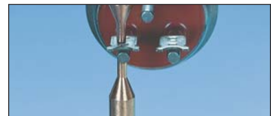
Weld electrical terminals to solid wire leads
