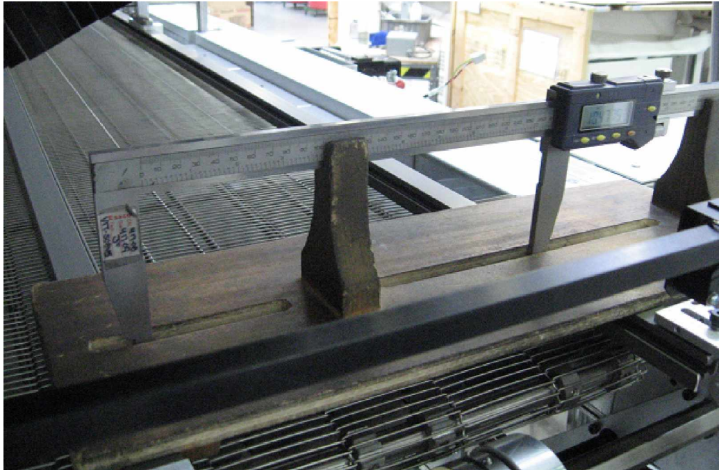
Digital calipers (in wooden support) measuring lane width at face above chain groove.
